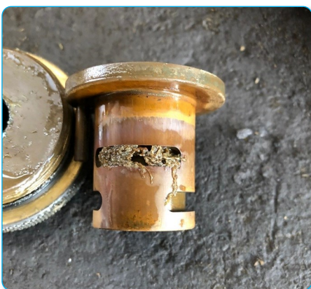
Nozzle clogged with biofilm
