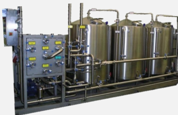
CIP system - note the many threaded connectors and shut-off valves.
