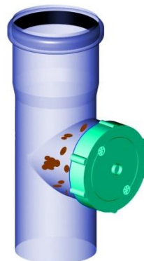
T joint with threaded connector following inadequate cleaning
