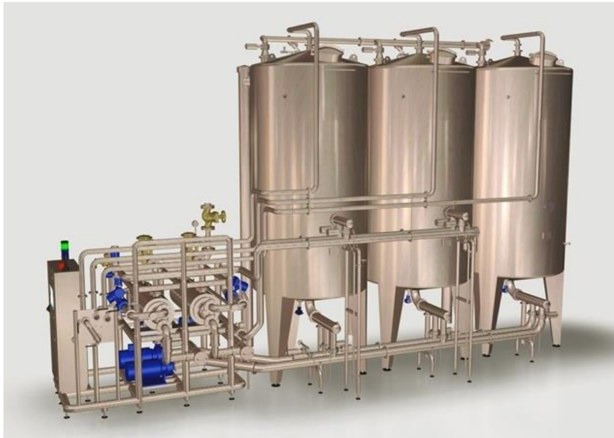
Simple CIP system with water/alkali/acid tanks, supply pumps, switchover plate and control system.
