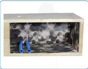
Cutaway model of a disinfectant foam application / pressing the foam into an underfloor structure after water damage
