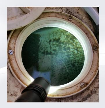
Biofilms quickly form on the surface in water tanks of ships, trains and mobile homes, etc.
